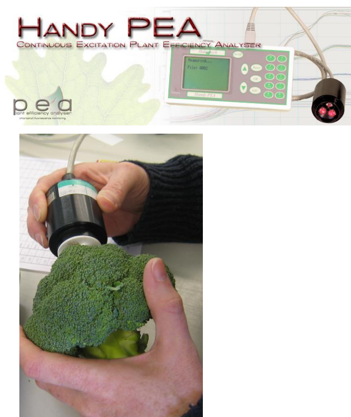
Figure 1. Handy Pea Chlorophyll fluorimeter (Hansatech Instruments Ltd, King's Lynn, UK). RH picture: Measurement from a broccoli head using an adapted leaf clip.
