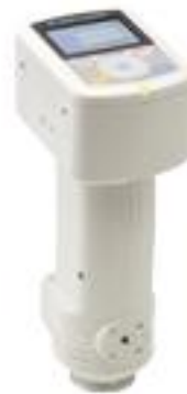
Figure 3. the L^* a^* b^* , colour space and Minolta colour meter used to measure machine colour values.
